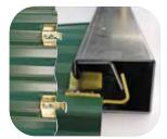
As wind blows against the 988WL, the curtain's windlocks engage with the door guide for a strong interlocking grip. This grip keeps the curtain securely in the quide.
